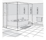
■ The safety rules define three volumes in a bathroom (see diagram 5). this unit must only be installed in volume 3 of the room so that the selector button (A) cannot be touched by anyone using the bath or the shower.
